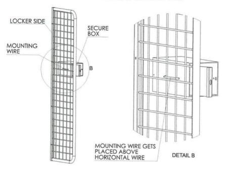
Open the SECUREBOX™ door and unthread the castle nuts from the mounting wire. Next follow the diagram below and position the mounting wire in the desired location you would like the box to be. Guide threaded ends through the holes in the box and thread the castle nuts back on and tighten with a 7/16" wrench.
