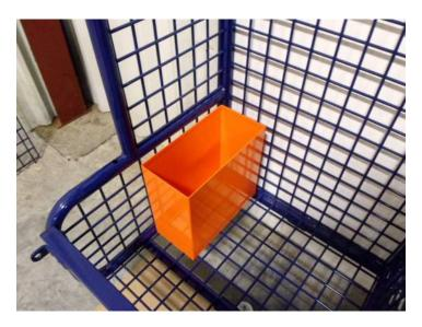
Step 2. Grab Gridiron Secure box mounting plate and place on the bottom of the locker (Make sure to line up holes of Secure box, and mounting plate) (See Photo) Next attach Secure box by using (4) threaded insert nuts and (4) insert bolts.
