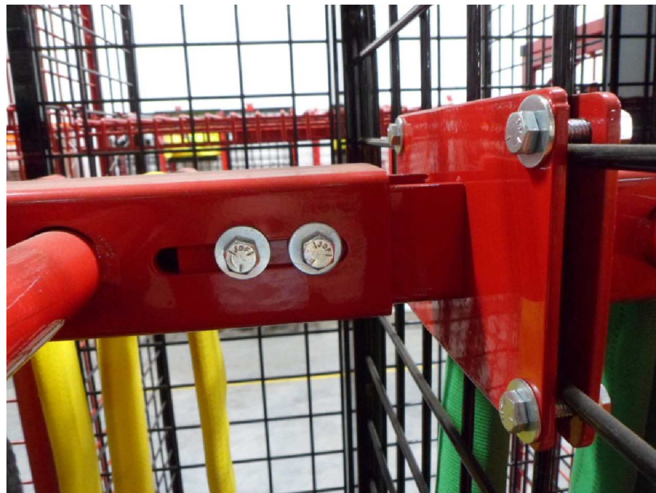
STEP 4: BOLT END JOINERS AND HOSE DRYER WELDMENTS TOGETHER AS SHOWN USING THE SUPPLIED 5/16-18 X 3/4" BOLTS AND WASHERS
