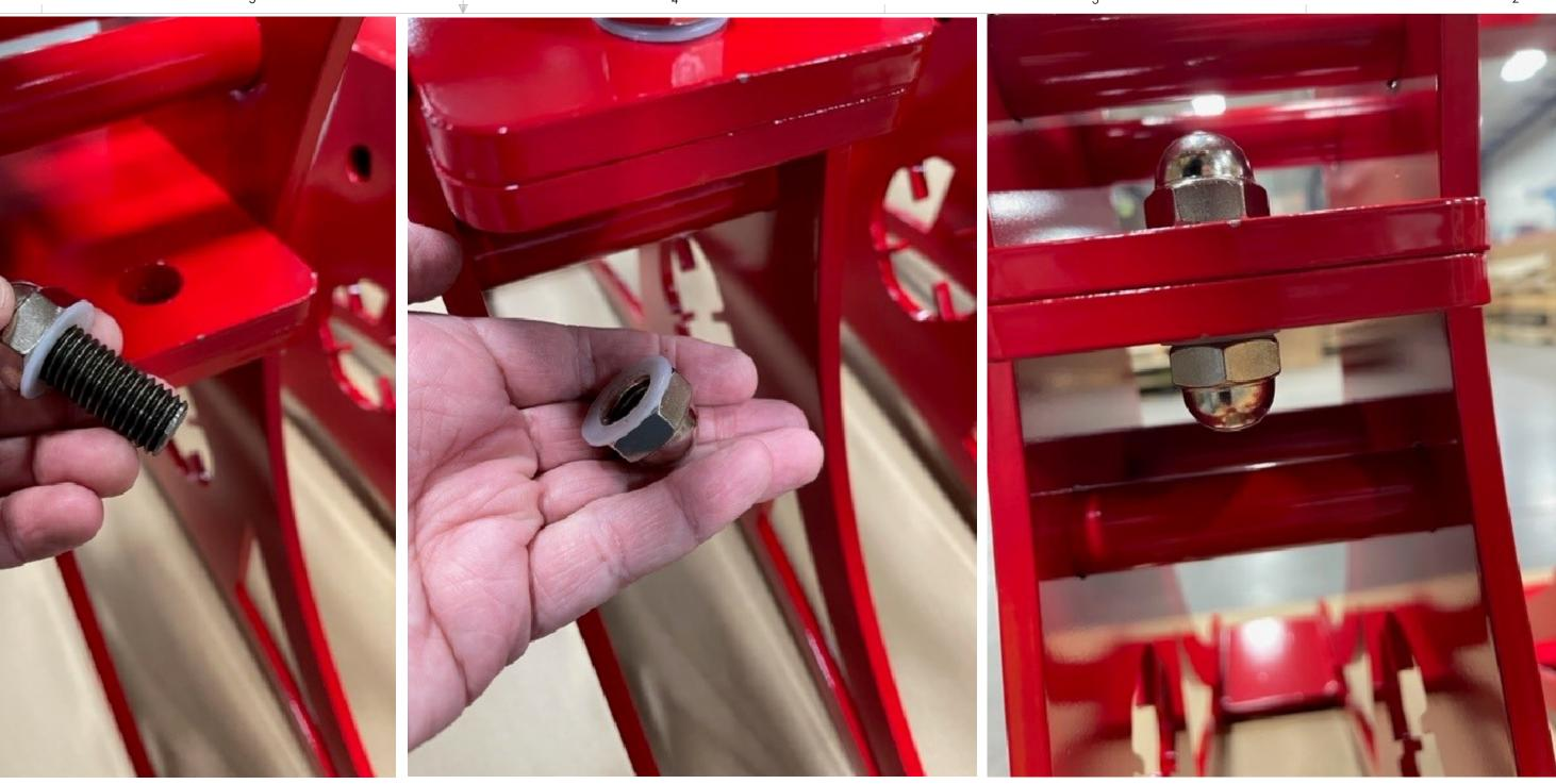
USE STUD, WASHER, AND CASTLE NUT TO JOIN BASE LEGS TOGETHER. USE A WASHER FOR EACH
