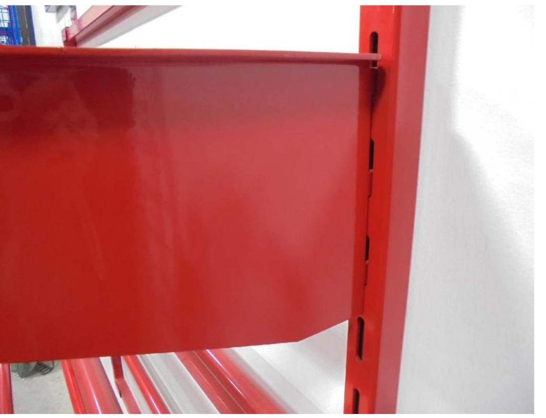
STEP 2: ONCE FRAME IS IN PLACE HANG YOUR SHELVES IN DESIRED LOCATION AS SHOWN ABOVE. THE THREE TABS ON SHELVES MATE TO THE SLOTS ON THE VERTICAL TUBES.
