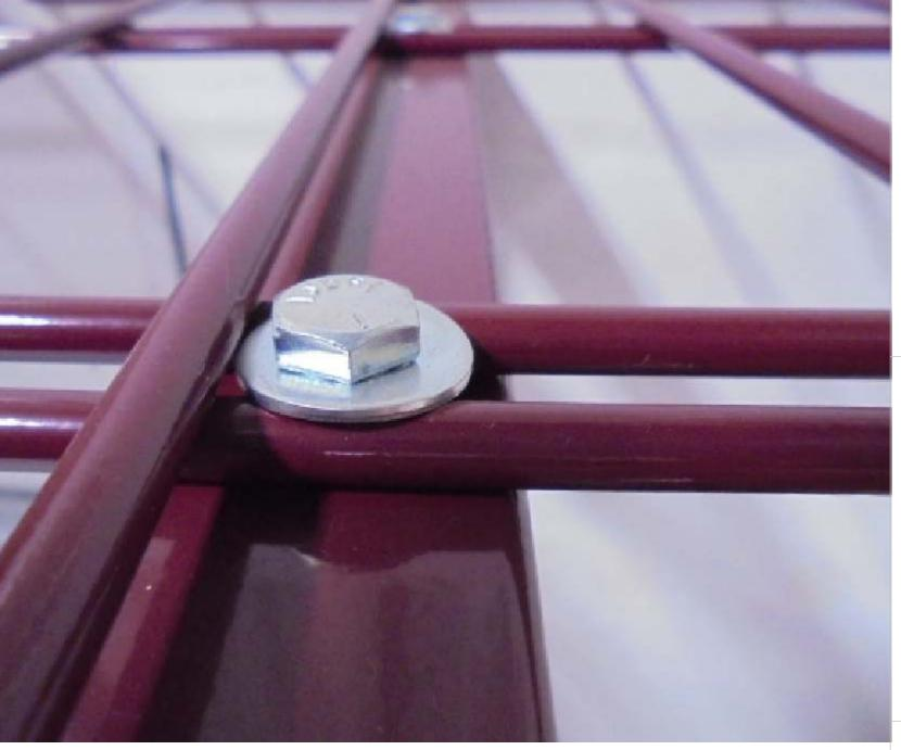
IMAGE SHOWS WASHER AND BOLT IN POSITION ON TOP. INSTALL HARWARE ON EACH BRACKET. USE WASHERS ON THE BOTTOM SIDE AND HAND START THE NUTS. ONCE SHELF IS POSITIONED THEN TIGHTEN HARDWARE.
