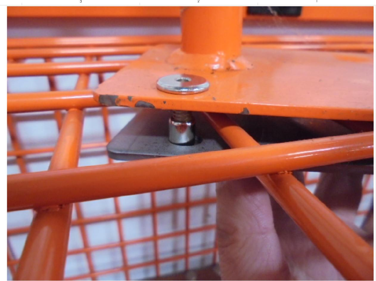
STEP 3: LINE UP BACKING PLATE AND INSTALL THE HARDWARE. TIGHTEN HARDWARE
