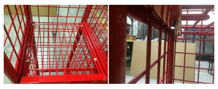
Step 5. Attaching locker doors to side tubes. First grab (4)  $.380 \times .750 \times .062$  nylon washers and place them on the tabs of the side tubes. (See photo) Next grab (1) locker door and (2) 1/2" shoulder bolts and insert bolts through door tabs and attach door to side tube. (See photo) Next, grab (4) acorn nuts and thread onto shoulder bolts. (See photo) now tighten hardware. <u>Do these steps for all doors.</u>
