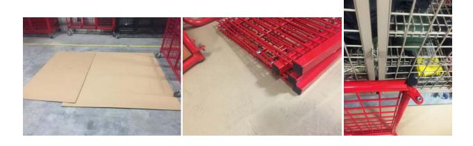
Step 2) Grab both 3-starts, and (6) 1/4-20x5-1/2" bolts, (6) 1/4" washers, (6) wedge nuts. Insert bolt and washer into locker channel and thread into wedge nut. Do these steps for both 3-starts. (Notice orientation of wedge nuts)
