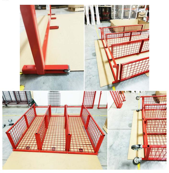
Step 3b. Lock rear casters, and stand locker system up. (Locking caster plates will keep lockers from rolling when standing up, also use safe lifting techniques to prevent injuries) Now once locker system is standing you can now install shelves. For bottom shelves you will be using 5/16-18 x 2-1/4" carriage bolts, washers, and 5/16-18 nuts, install these on front base tube only.
