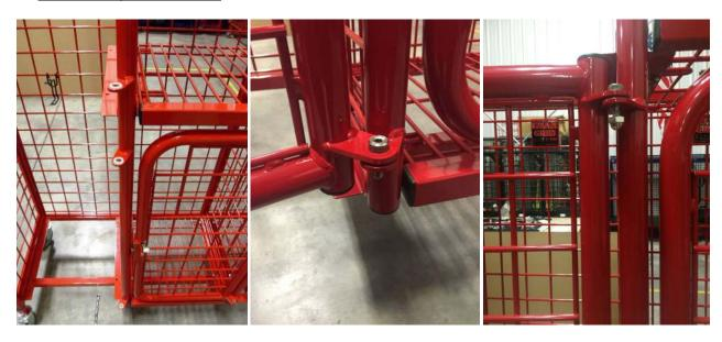
Step 6. Attach striker bolt. Per side, grab (2) striker bolts and thread into side tube, then tighten striker bolts (see photo).
