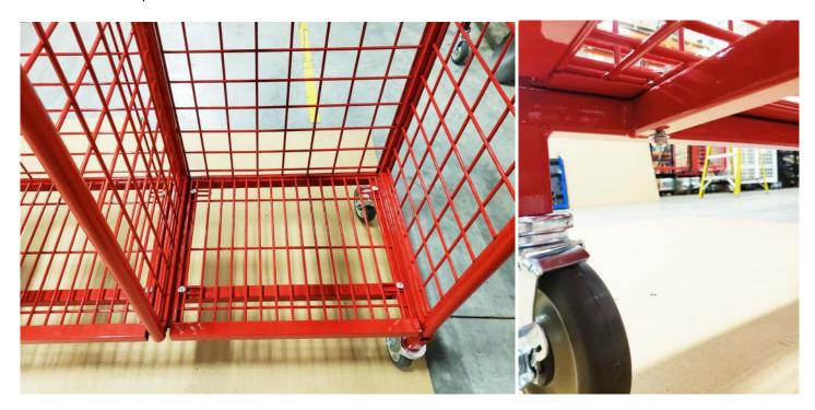
Step 4. Attaching shelves. Grab (1) shelf, (4) 1"x5/16-8 carriage bolts, (4) 5/16-18 nuts, and washers (not shown). Insert carriage bolt into shelf and through bracket, now thread on nut. Do these steps for all shelves. (There are (3) shelves per opening) Do not tighten hardware until all doors are installed. Leaving hardware loose will allow you some adjustability in the side panels for centering doors. Once your doors are centered you may now tighten hardware.
