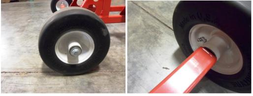
Step 2. Install Bearings to hose winder using (4) 3/8-16x3/4" flanged bolt and (4) 3/8-16 jam nut. See Photo. (Make sure to keep set screws facing inwards.) Do not tighten set screws at this time. Install lock nuts on bottom of bracket. See Photo.
