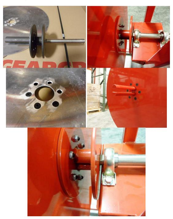
Step 4. Attach handle to hose winder bracket. See Photo. Next, install hose winder bracket to slotted plate holder bracket using (1) 5/16-18x2" bolt and (1) 5/16 lock nut. Note; the slotted hose winder bracket will have a pre-dilled hole for 5/16 bolt. See photo. Now tighten bolts.
