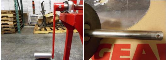
Step 5. Install nylon roller to hose winder frame by using 1/2"-13x8" and 1/2" jam nut. See Photo. Do not over tighten bolt.
