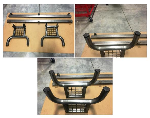
Step 2. Next, grab both long rectangle tubes and lay them so the (6) tabs are facing the floor. (See photo) Note: when laying these tubes down you will notice one tube will have (1) weld dot and the other tube will have (2) weld dots. (See photo) You must use a (1) and (2) dot tube for assembly, or the bench will not assembly correctly.
