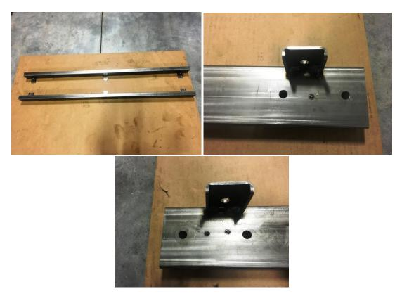
Step 3. Take both bench ends and slide channel into long tubes. (See photo) Next, flush up ends to long tube and insert (4) 5/16-18x3/4 bolts and (4) 5/16 washers per side. (See photo) **Note: Do not tighten bolts at this time.**
