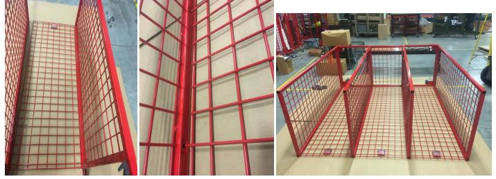
Step 5. Next, flush up the base to the side tube panels. (See photo) Next, tighten all 6-1/2" bolts and 5-1/2" base bolts. (See photo)
