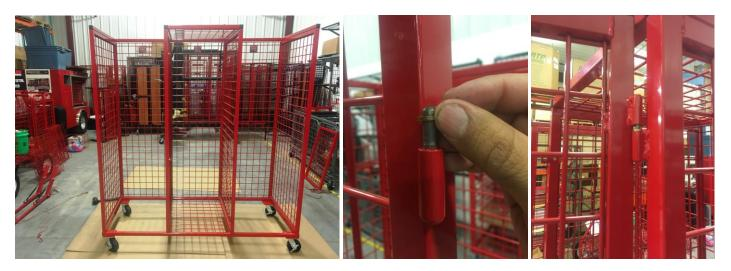
Step 9. Grab door latch (See Photo) (2) 1/4x20-3/8 button head screws, and attach to door. (See photo) Do not tighten hardware. Next close door to center door latch, now tighten hardware.
