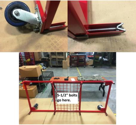
Step 3. Grab Sides and slide them just over the base channels (this will make installing back grids easier) (See photo) When laying out side panels make sure the punched holes are to the back of the base. Side panels should be placed in this order from left to right. Side panel, then side panel with hinges for doors, then side panel with hasp, then side panel. (See Photo)
