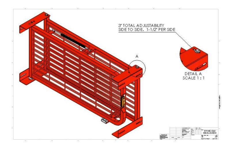
Thank you for the purchase of the Geargrid Swing Out Tool Grid. You should receive your tool grid fully assembled and ready for installation. Your tool grid has been fabricated slightly shorter than the clear open height to allow for flexibility in mounting. The width of the tool grid is adjustable. The diagram above shows the bolts to loosen if you need to adjust the width. Simply loosen and slide the mounting brackets out or in.
