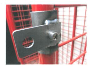
**4e.)** Install the wire latch assembly using the supplied 1/4" x 3/8" button head screws as shown below in the photo. Hand start the screws, shut the door to adjust position then tighten the screws.
