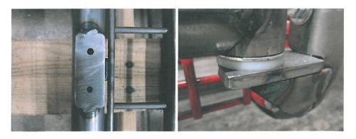
**4b.)** Install the supplied hasp drill fixture to the door plate as shown in the photo below using the 1/4" x 3/8" button head screws.
